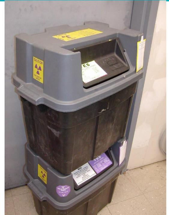
Above is a standard waste container labeled for radioactive waste. The solid waste from  $^{117m}\text{Sn}$  contains such a small amount of radioactivity that the container is not required to be shielded.
