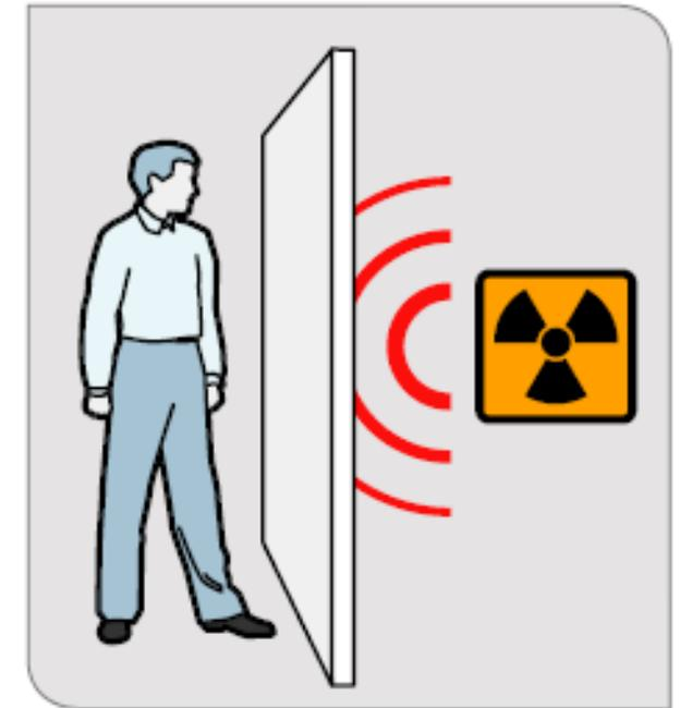
**Shielding:** If you have a thick shield between yourself and the radioactive materials more of the radiation will be absorbed by the thick shield, and you will be exposed to less.
